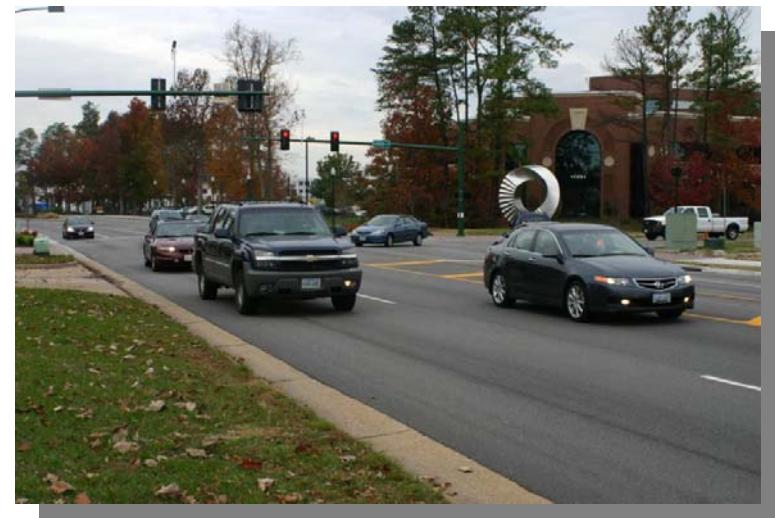
*Canon Blvd at Thimble Shoals Blvd is currently operating at LOS F during the PM peak hour. With optimized signal timings, the intersection will operate at LOS C.*
