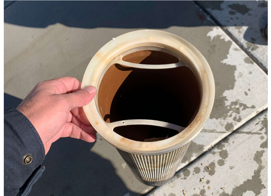
Filter bags within a few weeks of operation
