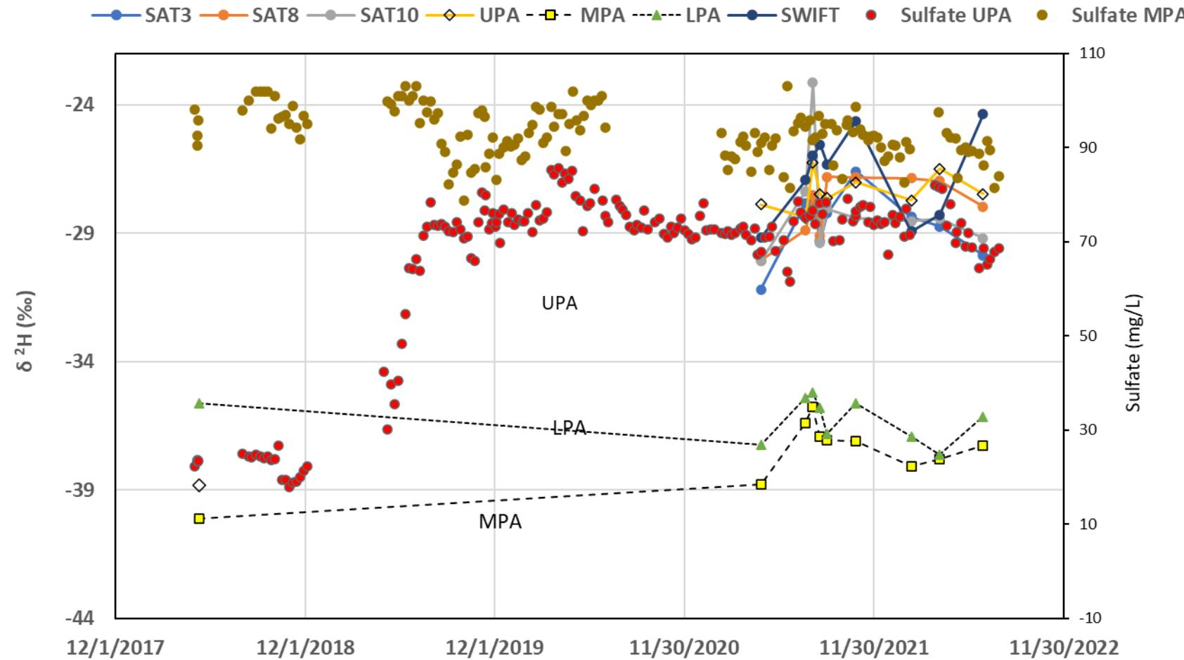
In MPA, sulfate shows less variation consistent with MPA isotope values.
