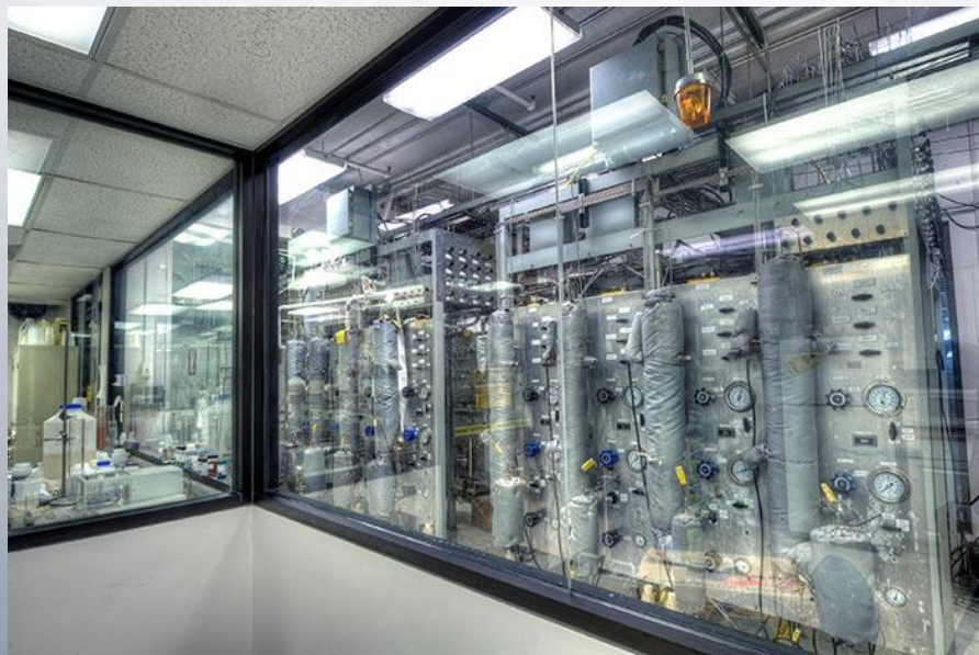
Laboratory scale reactor stations that can be configured as fixed-bed, trickle bed or continuous stirred tank reactors (CSTR).
