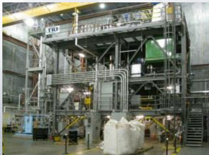
Full commercial scale tubular (fixed-bed) FT reactor) at TRI's demonstration facility in Raleigh Durham, NC.
