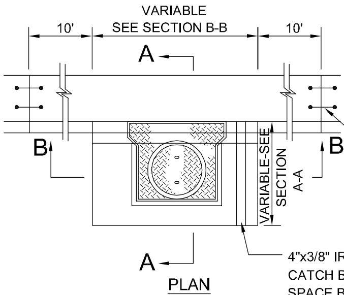
(2)-24" #4 DOWELS, PLACED 2" ABOVE GUTTER BOTTOM AND CENTERED AT JOINT (TYP. EACH SIDE)
