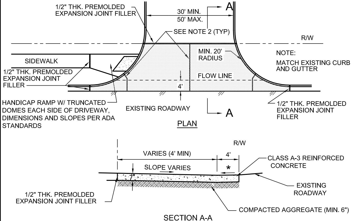
\* TO MATCH 24" CURB & GUTTER, SLOPE = 1" : 32"
