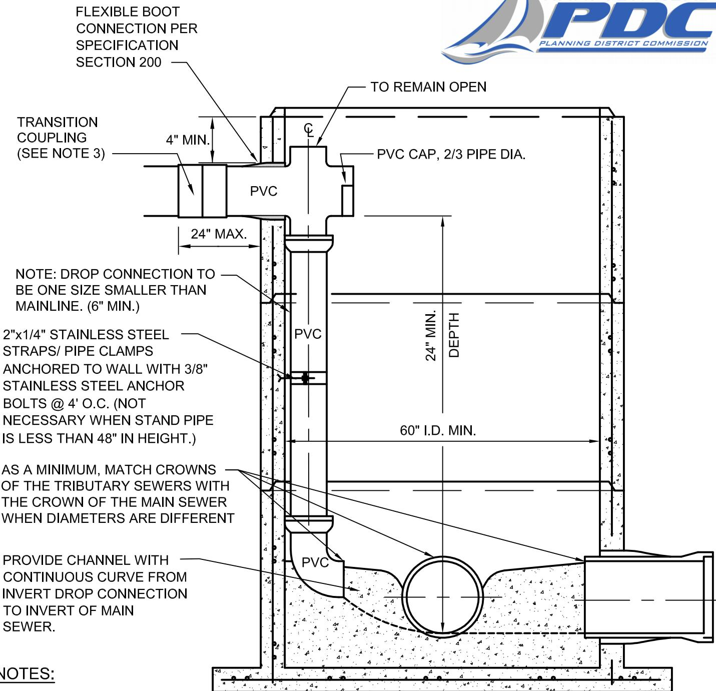
1. INTERIOR DROP TO BE USED IN NEW MANHOLES.
